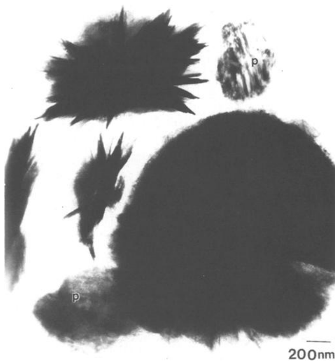
Fig. 3. Bright field transmission electron micrograph of the activated catalyst showing rosette-shaped clusters and one of the less common individual isolated platelets.
